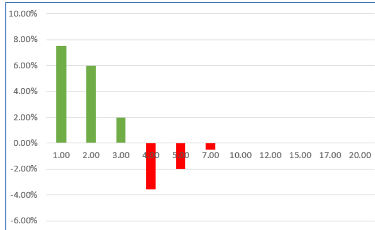
Figure 19. The difference in energy source level with and without sleep mode considering different workloads
