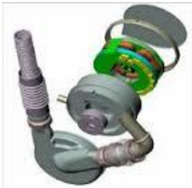
Figure 1.8 HeartMate III centrifugal pump. From: Cardiol Clin 2011; 29(4): 559-582 and https://www.lvad.nl/en/heartmate-3/
