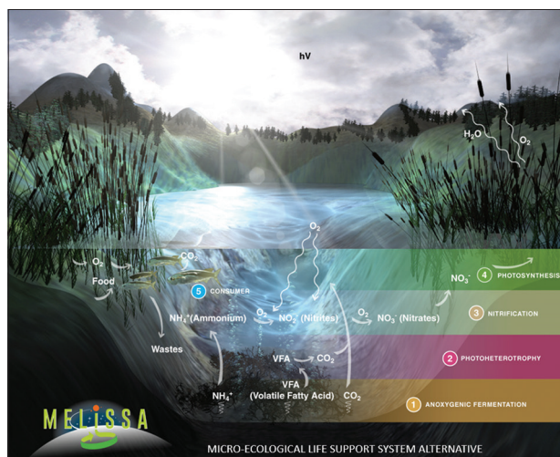
Figure 3. Micro Ecological Life Support System Alternative program (MELiSSA) proposes regenerative life support technologies to produce food, recovery of water, and atmosphere regeneration, together with waste reclamation. Source: MELiSSA Foundation
