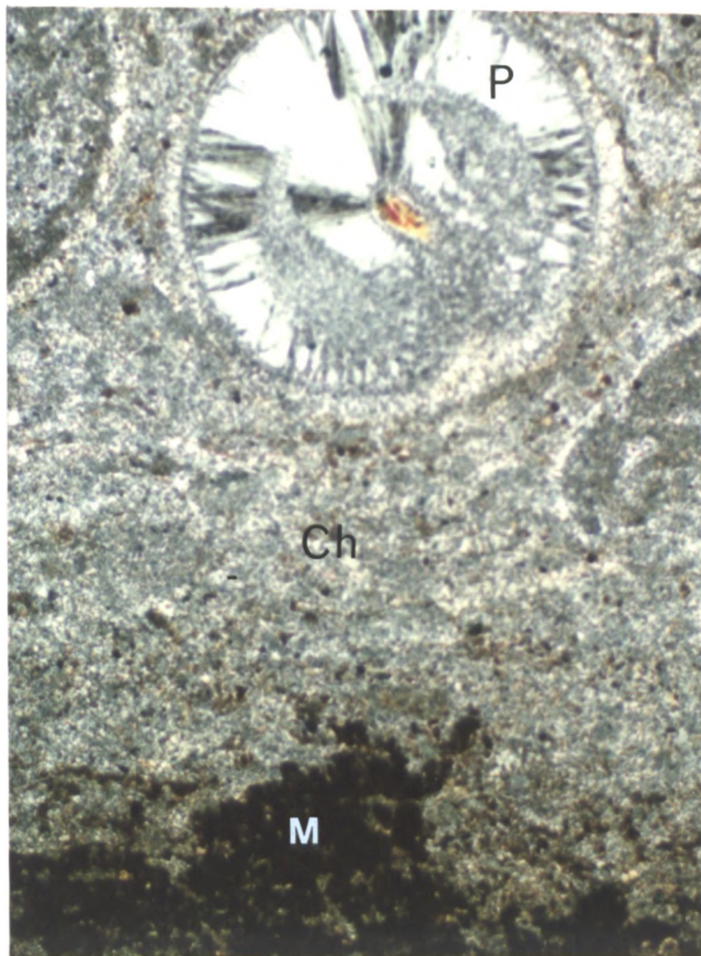
FIG 3.58 Thin section of chert nodule within lacustrine limestone. Planorbis gastropods (P) replaced by silica enclosed within micro-crystalline chert (Ch), which replaces micritic limestone (M). Bedding is horizontal. X 10.
