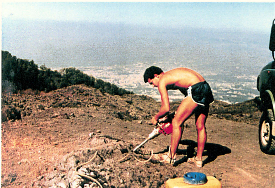
Figure 2.1 Drilling a core from the 1944 lava flow on Mount Vesuvius.
