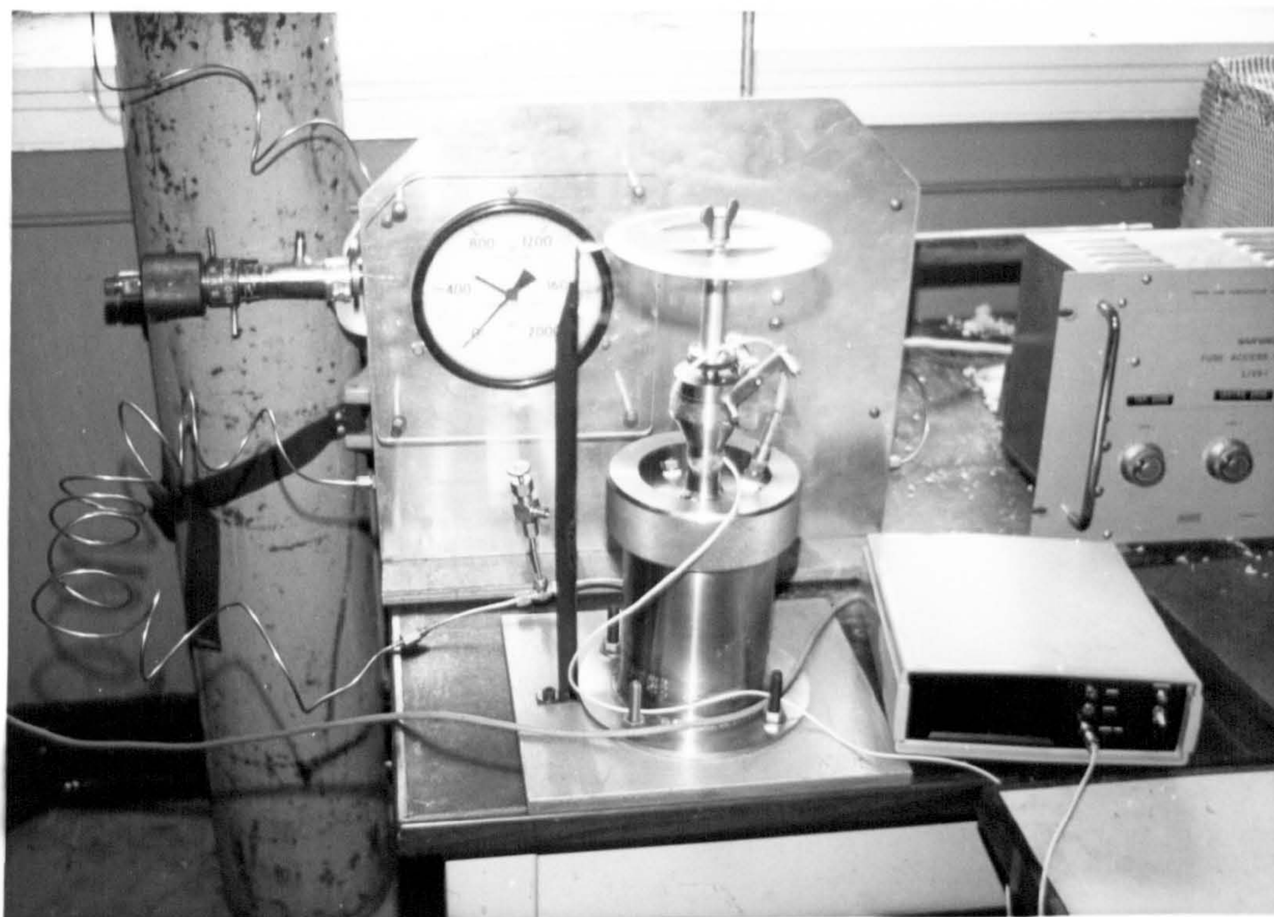
Fig 5.5 4-point bend test equipment
