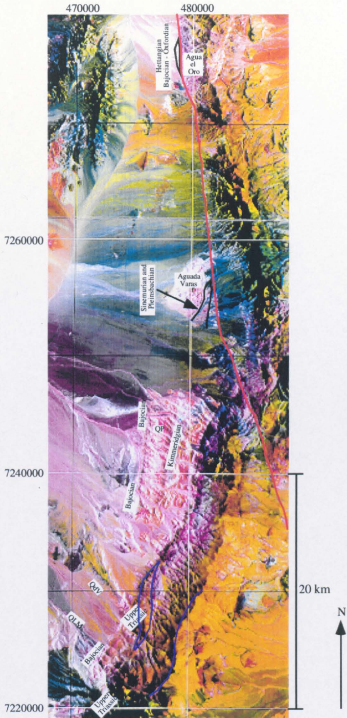
Figure 2.1.5 Satellite image showing Jurassic outcrops along the western flank of the Domeyko. QP, QdV and QLM indicate Q. Profeta, Q. del Viento and Q. Las Mulas respectively. The deflection of the main ridge and s-shaped body of La Tabla Formation have been outlined in blue to aid their location. Closer inspection of this deflection is visible in Figure 2.1.2. The outcrop limits are drawn in for Agua el Oro and Aguada Varas.
