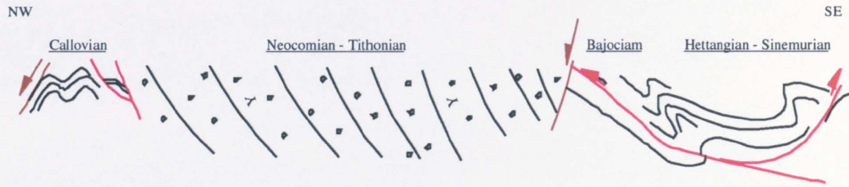
Figure 2.1.6 (a) A schematic cross section of Q. Las Mulas. The sense of movement on the fault juxtaposing Bajocian and Neocomian sediments is inferred from stratigraphy. A small rhyolite intrusion occurs along this fault and is cut by the normal fault, as shown on Fold out 2.1, but has been omitted here for clarity. The sense of movement between the Neocomian and Callovian sediments is unknown.
