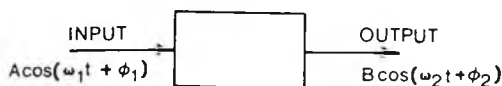
Figure 4. Entrainment of wakes from idealised insertion of sinusoidal input to upstream non-linear oscillating blade aeromechanical system. Resulting entrainment is stable if \omega_1 = \omega_2 and \psi_2 constant; metastable if \omega_1 = \omega_2 but B and \psi_2 may vary; unstable if \omega_1 \neq \omega_2 necessarily and B, \psi_2 are unstable.
