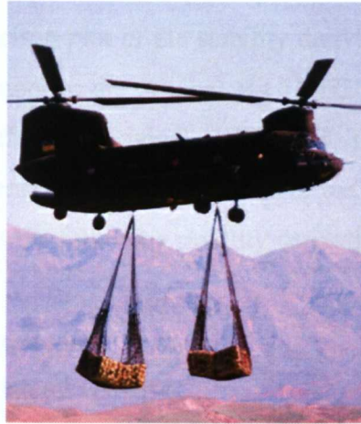
Figure 2.3: CH-47 tandem rotor helicopter with dual hook suspension [38]
