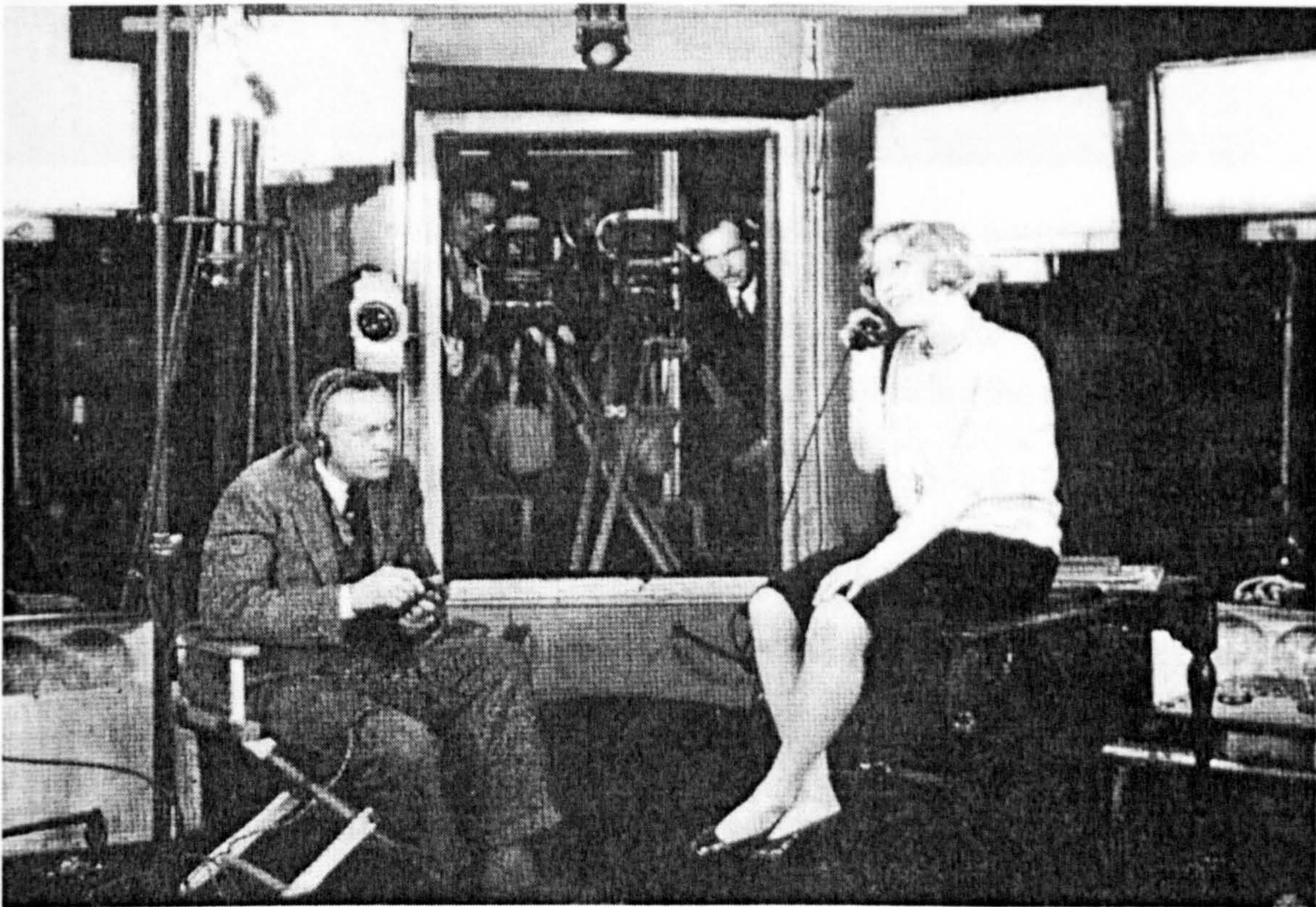
Figure 9.4 A sound proof booth (with double or triple gazing) used in early talking pictures made increases in camera to subject distances inevitable, and close-up photography very difficult as this simulated scene shows. (The Movie, encyclopaedia p.22 Orbis Press 1982)
