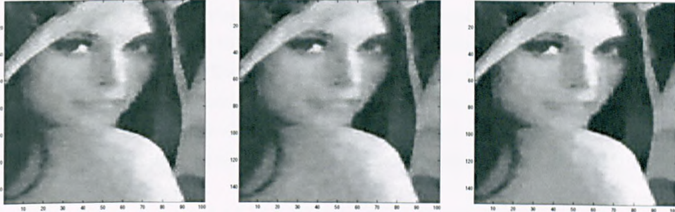
Figure 6.7: Close up of Lenna Image recovered using model 3 (left) and model 4 (centre), with TV result (right) for comparison, notice the reduction in staircasing on the face and shoulder
