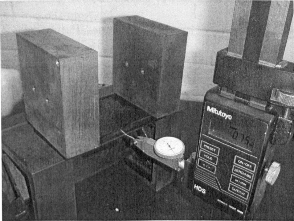
Figure 3.24 Measurement of the mid-point deflection of the blast-loaded panels.
