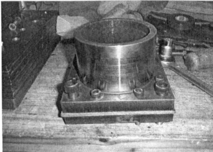
Figure 3.21 Photograph of the test plate and the clamping rig.
