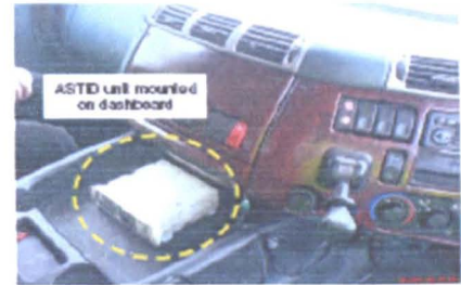
Figure 2. Shows the ASTiD system mounted on the dashboard of a vehicle.
