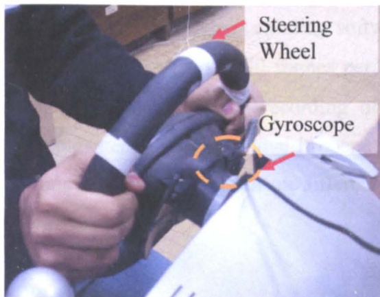
Figure 3.4.2.1 – Gyroscope installation on a laboratory based steering wheel
