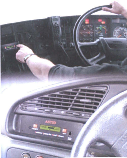
Figure 3.2.3.2 – Showing an ASTiD unit installed onto the universal dim slot of the dashboard. [Pernix, 2005]
