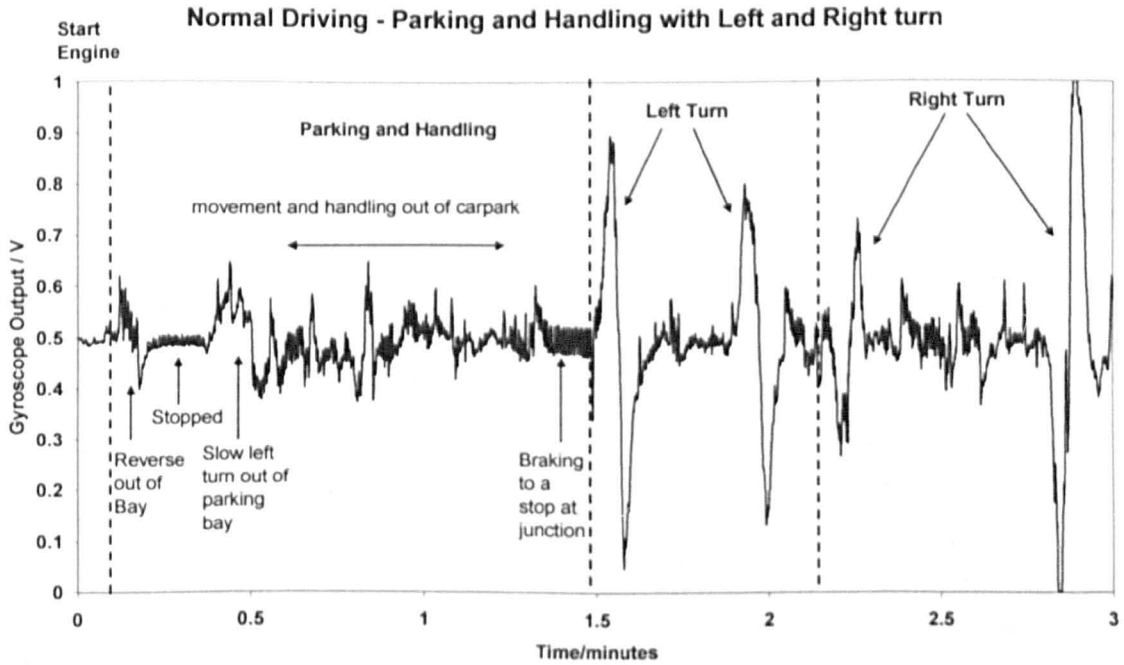
Figure 5.3.2.1. Gyroscope output showing signal features of 2 different manoeuvres: Parking and Handling (0-1.5min) & Left and right turning (1.5-3min)
