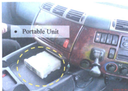
Figure 3.4.1.1 –Implementation of the gyroscope system on the dashboard of a vehicle [Koh et al 2007]
