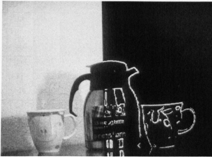
Figure 8-29 Sobel edge detector image – mugs and jug (threshold=60)
