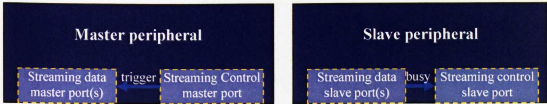
Figure 6-9 Master peripheral and slave peripheral with streaming control feature
