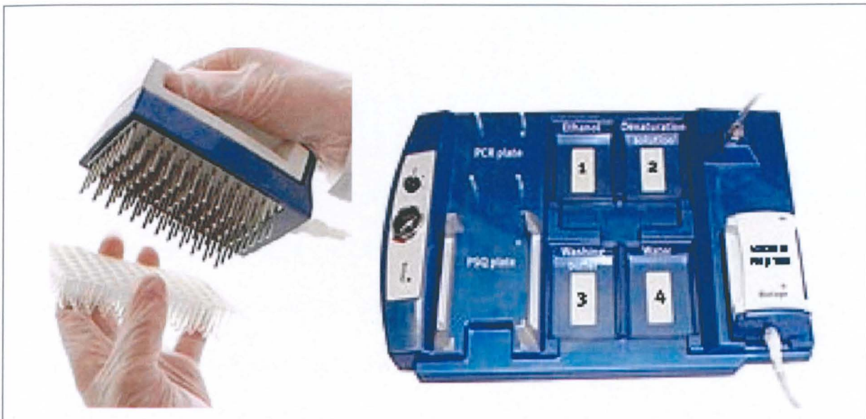
Figure 4.2.8.1. PyroMark Vacuum Prep Tool and PyroMark Vacuum Prep Worktable (Qiagen) for preparation of the pyrosequencing template. Biotinylated PCR products immobilised on streptavidin-sepharose beads which are consequently collected on the probe tips of the vacuum tool. Washes with 70% ethanol (position 1), 0.2M NaOH (position 2) and 10 mM Tris Acetate PH 7.5 (position 3) results in the desired single strand pyrosequencing template. Trough no 4 contains ddH 2 O for the final wash of the tool after use. ( http://www.pyrosequencing.com/DynPage.aspx?id=7267 ).
