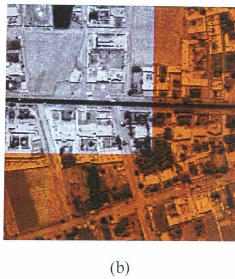
Figure 4.4 Example of shift registration images: (a) synthetic image registration without cloud (b) registered image overlapped with the reference image.
