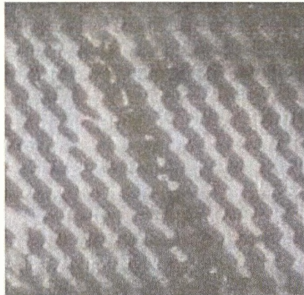
Figure 4.82 Surface finish due to mechanical failure of the composite at x2 magnification
