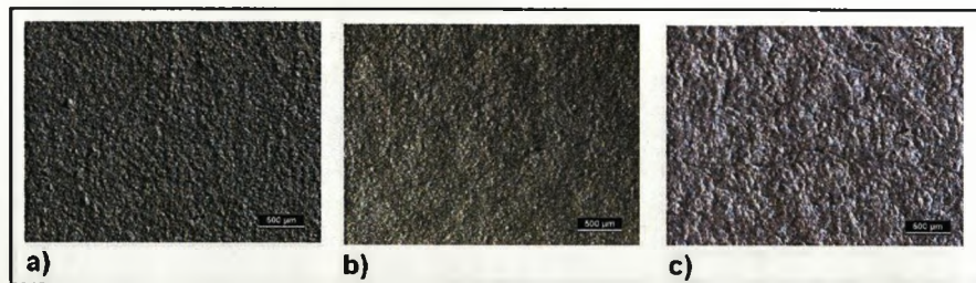
Figure 4.2: Micrographs for a) thin, b) thick and c) saturated graphite application methods taken at x5 magnification
