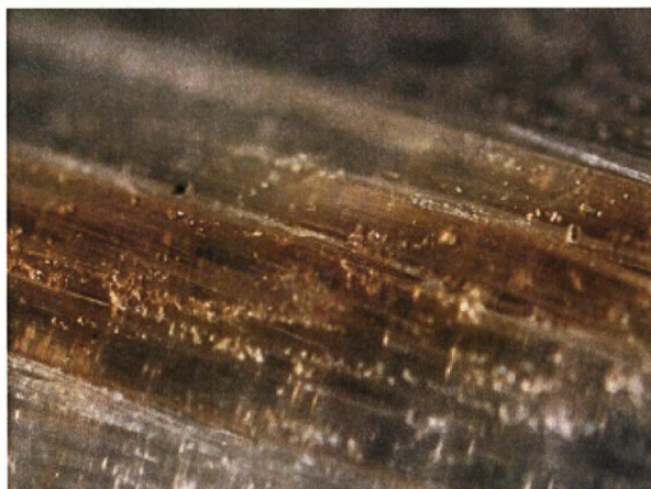
Figure 4.85 Detail of burning of matrix at x5 magnification
