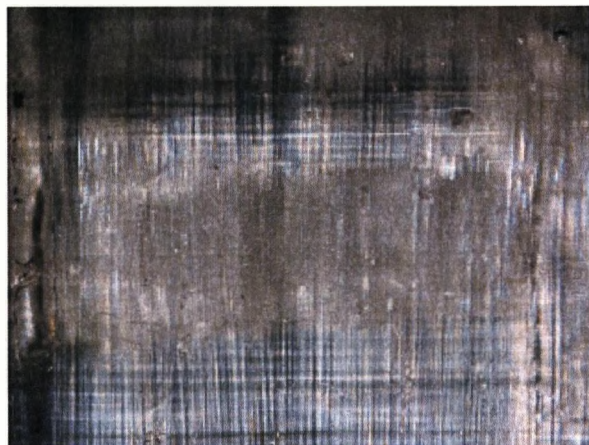
Figure 4.87 Image of failure of fibres in 1:1 90° GF FML (fibres orientated vertically in image) at x10 magnification
