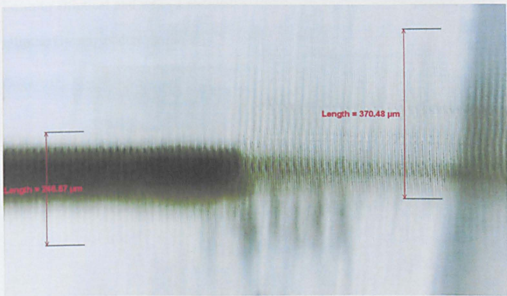
Fig. 7.2-2: A modification thickness of 247 \mu\text{m} (left) produced without beam shaping, and a modification thickness 370 \mu\text{m} (right) produced with beam shaping.
