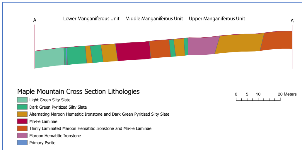
Figure 42. Generalized cross section at Stop 7 showing the lower, middle, and upper manganiferous units.
