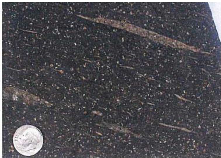
Figure 2: An example of Traveler Rhyolite (Black Cat Member). Flattened pumice (tan areas) highlights the compaction foliation of this welded tuff. Phenocrysts appear as white specks. Photo modified from Rankin and Caldwell (2010).
