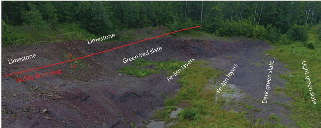
Figure 35. Birdseye view of the Dudley pit (south pit) from a drone. Facing south. U – upthrown, D – downthrown.
