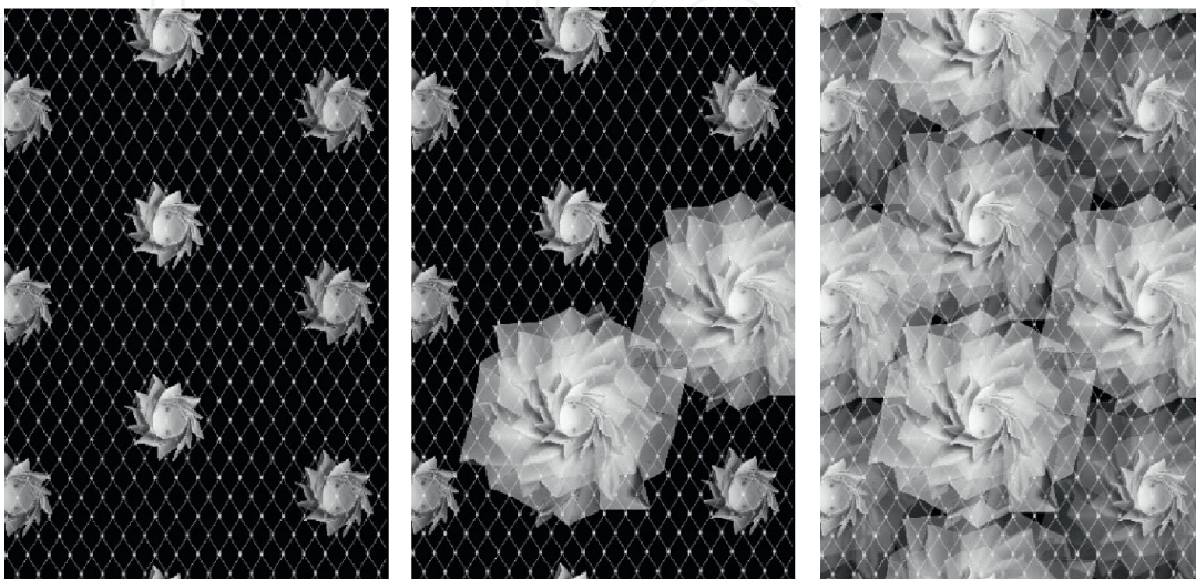
Figure 17. Visualization of PAOSS in un-activated closed state (right), targeted partial glare protection state (middle), and full-surface shading state (left) © C. Eisenbarth/ILEK.
