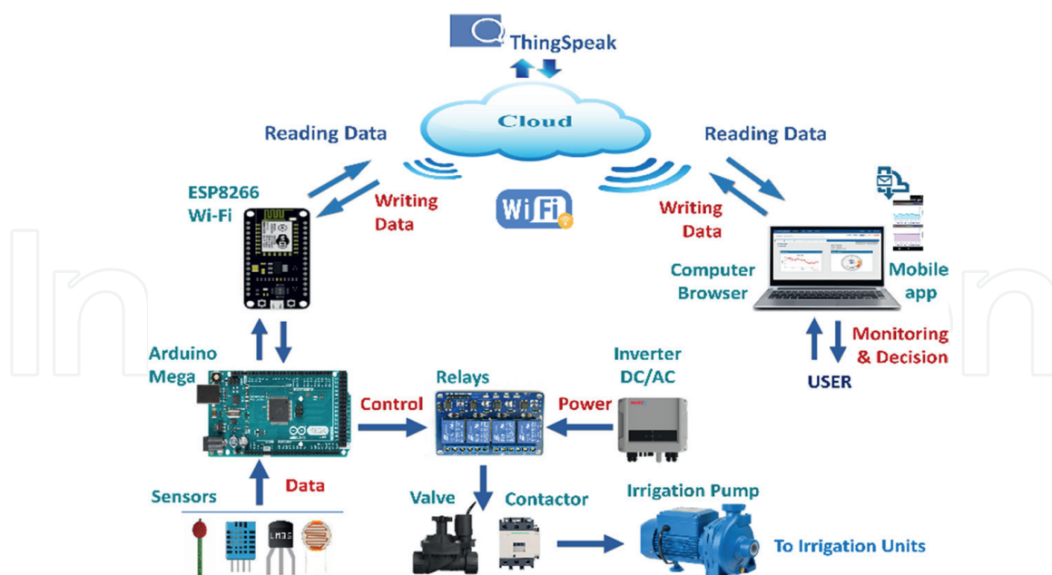
Figure 2. A schematic diagram for the IoT-based control system for a smart subsurface irrigation for enhancing irrigation management of date palm.
