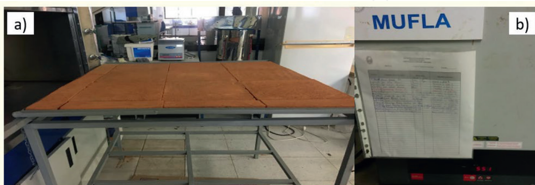
Figure 3. (a) Catalyst support and placing clay plates on the FFPR, (b) calcination process, observing the porosity and homogeneity on the surface of the plate.
