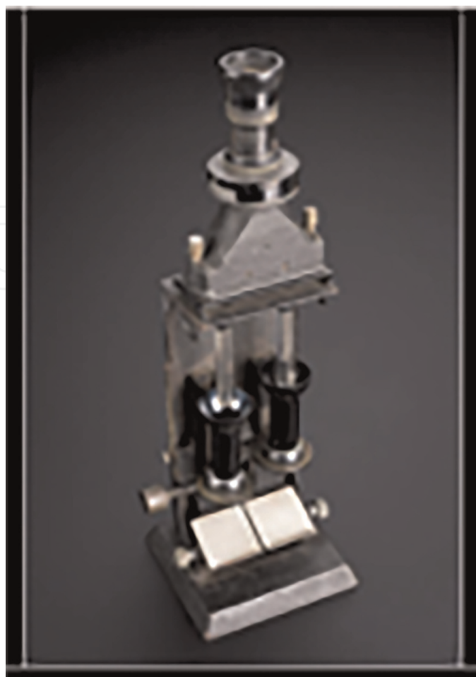
Figure 2. Duboscq colorimeter, by F. Hellige and Co., Freiburg, Germany, 1901–1914.
