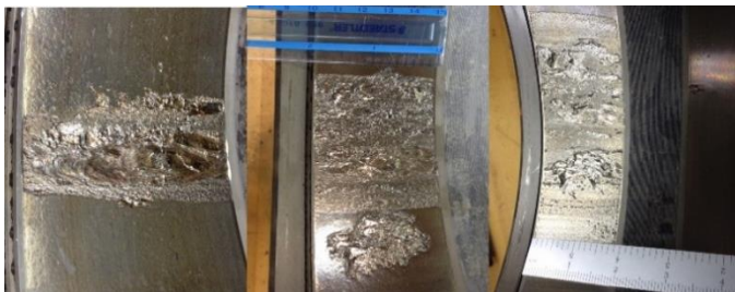
Figure 5. Spall growth in a bearing outer ring (cup) under continued operation (increasing mileage left to right).
