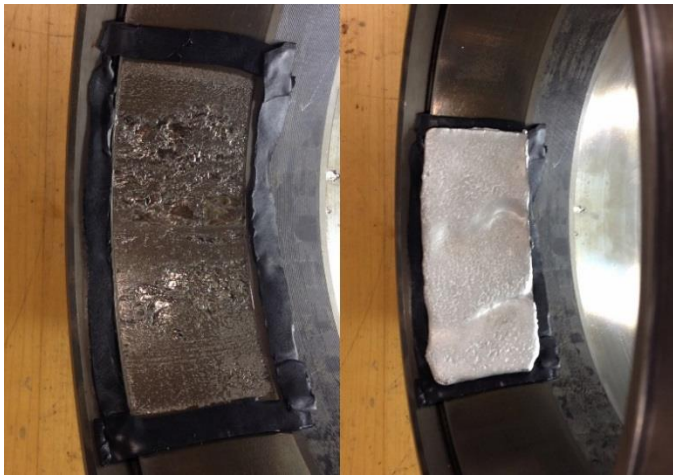
Figure 4. Bismuth casting procedure. Spalled surface with tacky tape (left); Bismuth alloy cast in place (right).
