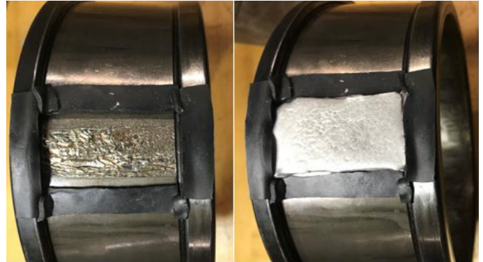
Figure 5. Casting procedure using Bismuth; (left) spalled surface outlined with tacky tape; (right) Bismuth alloy cast
