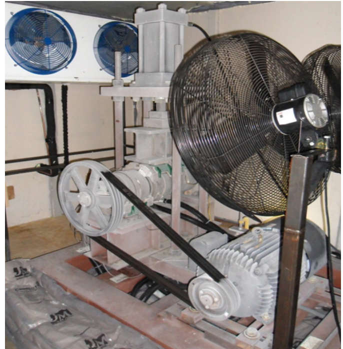
Figure 2. Older design of the four-bearing tester housed within the environmental chamber showing tester at -40°C
