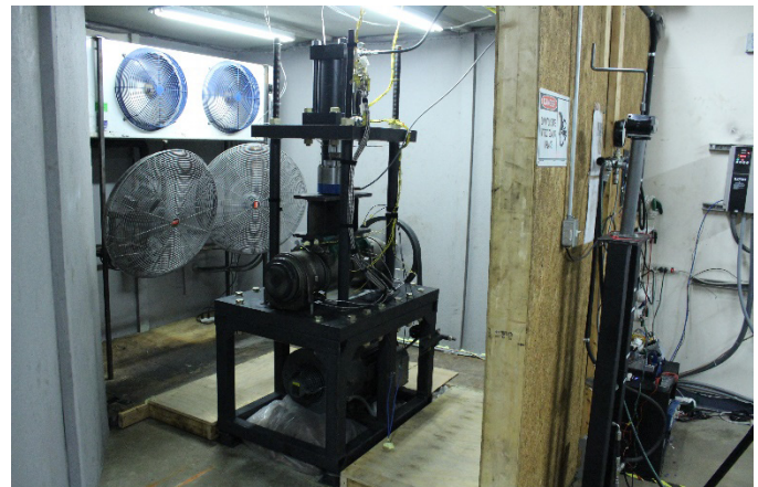
Figure 3. New design of the four-bearing dynamic tester housed within the environmental chamber
