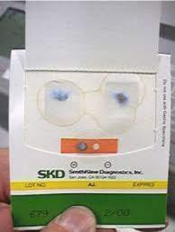
Both square test areas in the upper area of the card show the intense blue color of a positive result. The lower two smaller circular areas on the orange stripe are analytical control reactions, positive on the left and negative on the right, that help assure that the card and developer bottle have been maintained in proper conditions and have not been damaged before the test is performed.
