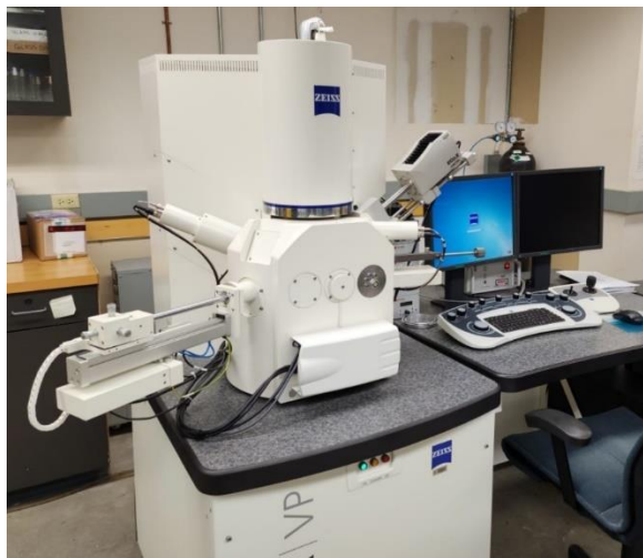
Figure 7: Image of Scanning Electron Microscope (SEM) machine and Energy Dispersive X-ray Spectroscopy (EDS).
