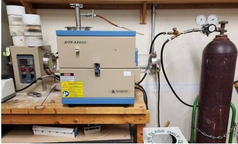
Figure 6: Image of tube furnace.
