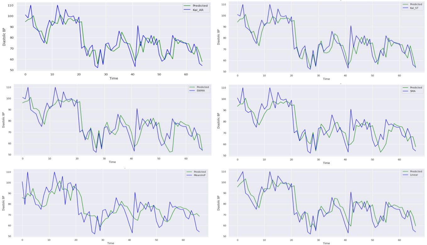
Figure 15: Prediction performance of LSTM in Kal AR (top left), Kal ST (top right), EWMA (middle left), SMA (middle right), mean (bottom left), and linear interpolation (bottom right) imputed dataset at 10% missing data rate.
