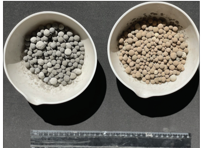
Figure 5: Difference in appearance between (left) cold bonded and (right) sintered pellets
