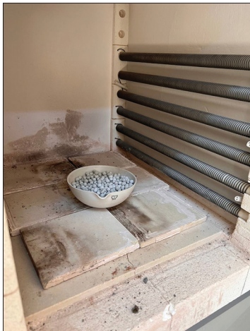
Figure 4: Sintering the pellets at 900°C
