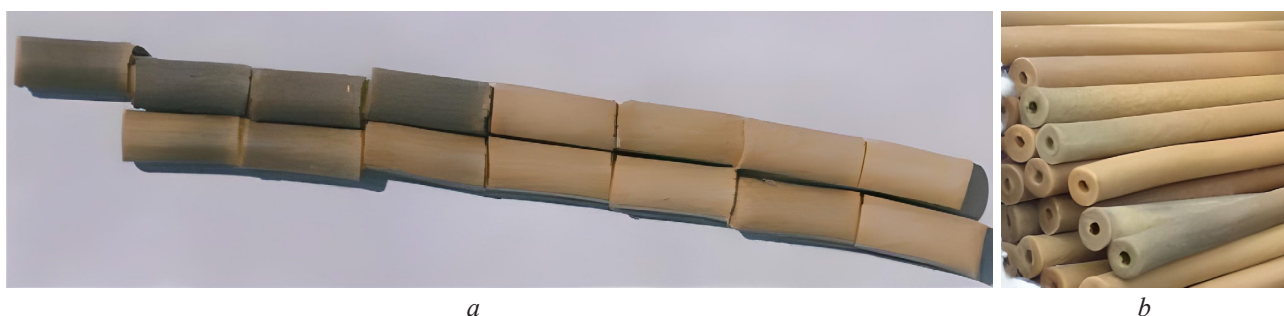
Fig. 2. Samples of 4Zh40 tank shot charge gunpowders after long-term storage: a – seven-channel; b – single-channel
