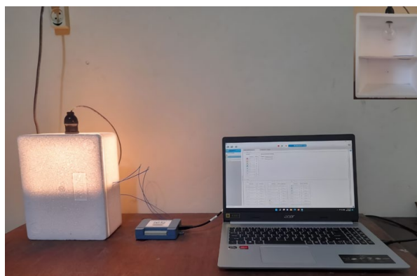
Fig. 12. Equipment to test the thermal performance of PCM composite
