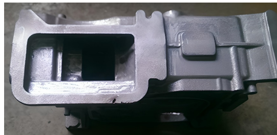
Fig. 2. The casting product with a porosity at the position of water tank
