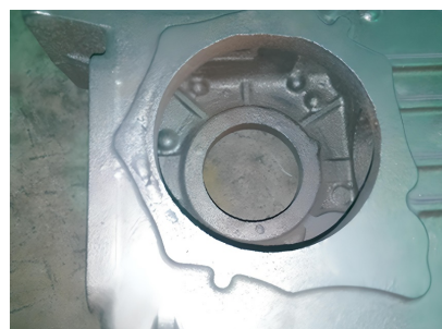
Fig. 4. The casting product with shortage of fill material
