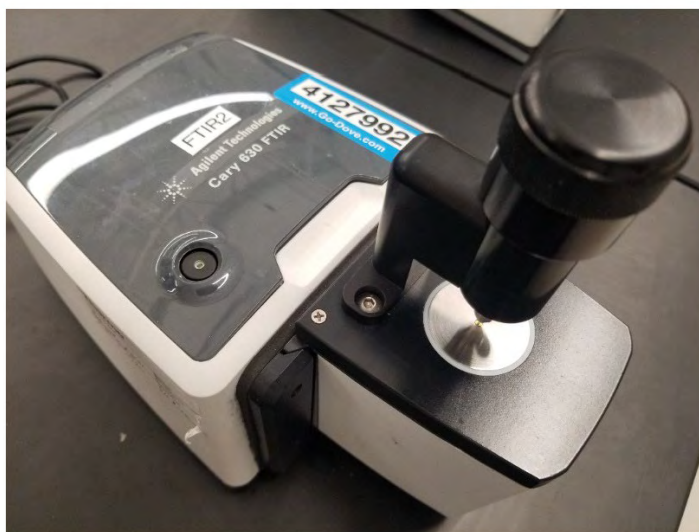
Figure 14. FTIR model: Agilent Cary 630 FTIR spectrometer with Diamond ATR.
