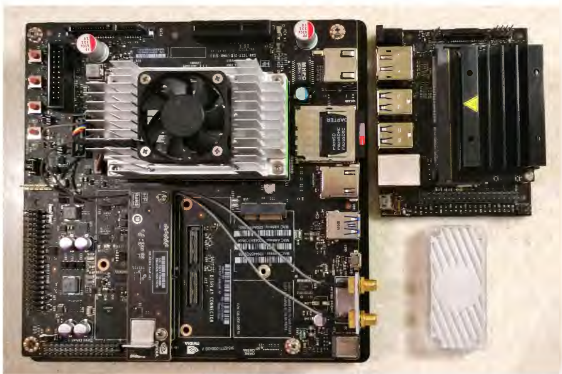
Fig. 3.4. Left: Jetson TX2, Right (Top): Jetson Nano, Right (Bottom): Google Coral TPU USB Accelerator
