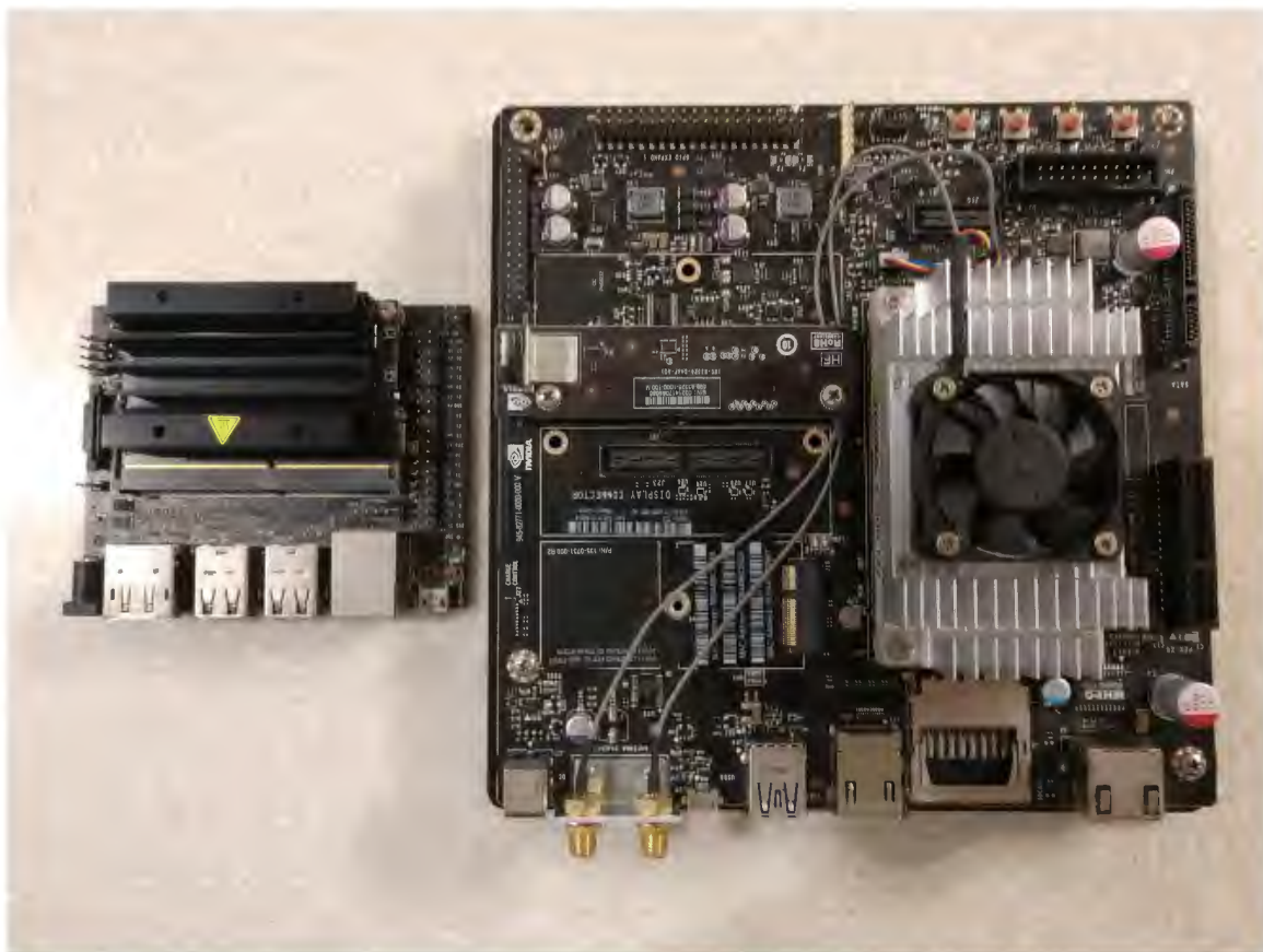
Fig. 4.4. NVIDIA Jetson Nano (left) and NVIDIA Jetson TX2 (right)
