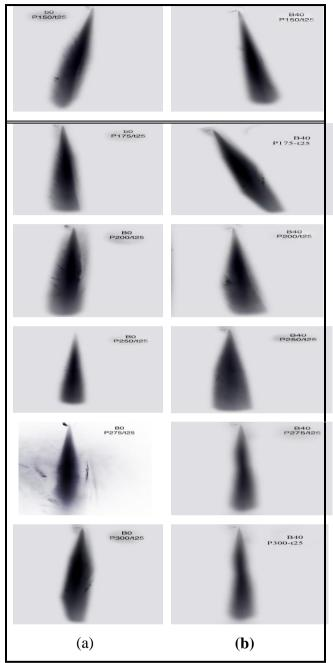
Figure 4: (a) Spray characteristics for B0 (b) B40 under injection pressure (150 bar to 300 bar) and ambient temperature 25 °C
