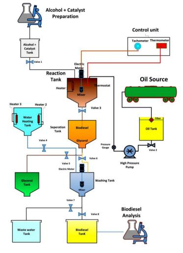
Figure 2: Schematic diagram for production process from WCO biodiesel
