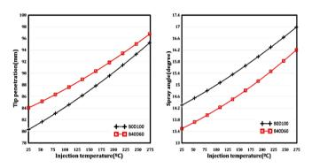
Figure 7: Effect of Injection temperature on tip Penetration and spray angle
