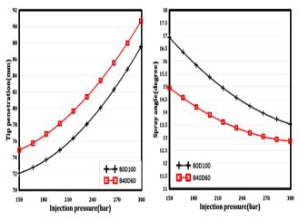
Figure 6: Effect of Injection Pressure on tip Penetration and spray angle
