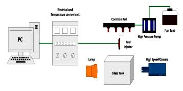
Figure 3: Experimental setup for study spray characteristics
