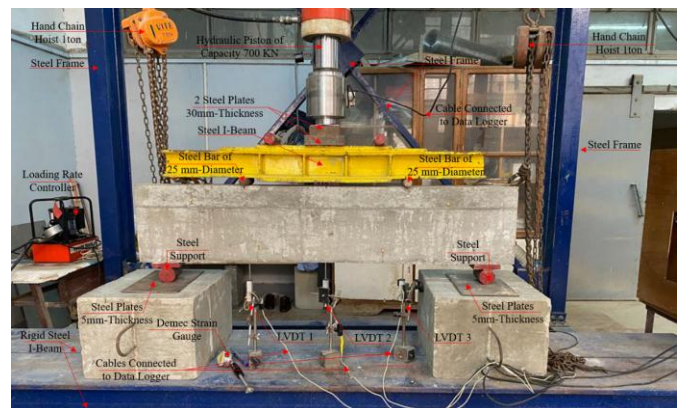
Figure 10. The test setup of beam specimens.
