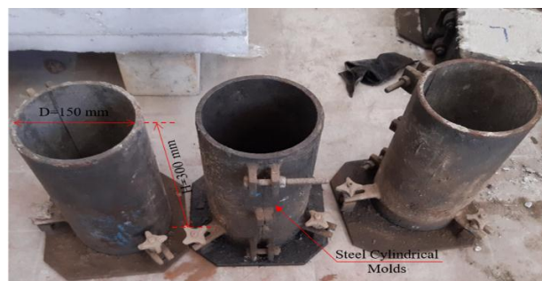
Figure 6 (c). The preparing of cylindrical concrete specimens.
