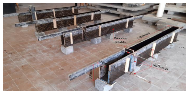
Figure 6 (d). The preparing of concrete beams specimens.
