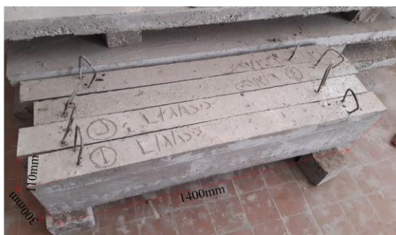
Figure 8. The reinforced concrete beams specimens after hardening. All beams are 110 mm wide, 300 mm deep and 1400 mm span.
