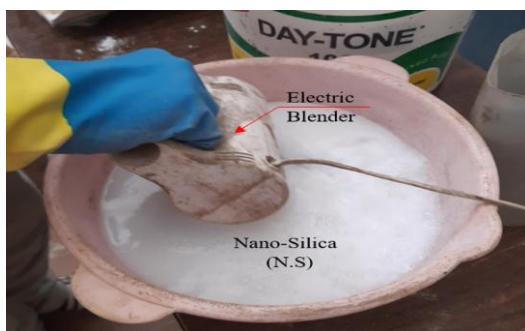
Figure 6 (a). Dispersion of Nano-Silica (NS) particles in the mixing water.
