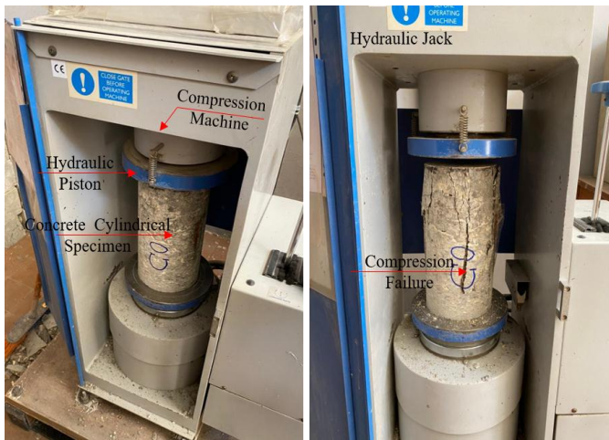
Figure 7. The compressive strength test according to ASTM C39/C39 M-21.
