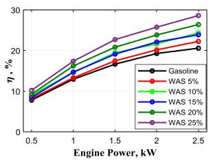
Fig. 5: Comparison of overall Efficiency for different gasoline/WAS blends at different power of an engine operating at a constant speed of 3000 rpm.
