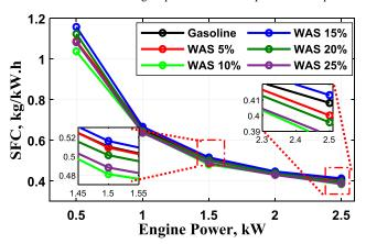
Fig. 4: Comparison of Specific fuel consumption for different gasoline/WAS blends at various engine power at constant speed 3000 rpm.
