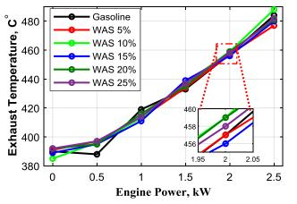
Fig. 6: Comparison of the exhaust temperature for different gasoline/WAS blends at various power of an engine running at a constant speed of 3000 rpm.
