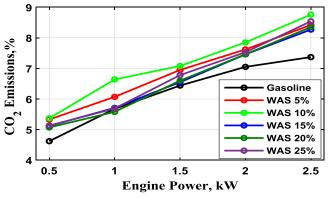
Fig. 8: Variation of the Co2 emissions with engine power for different gasoline/WAS blends at engine constant speed of 3000 rpm.
