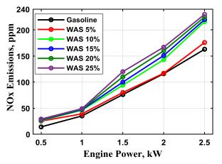
Fig. 10: Variation of the NOx emissions with engine power for different gasoline/WAS blends at engine constant speed of 3000 rpm.
