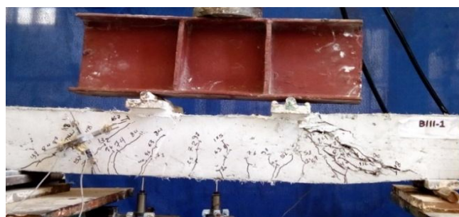
Fig. 9: Final crack pattern of beam BIII-1.
