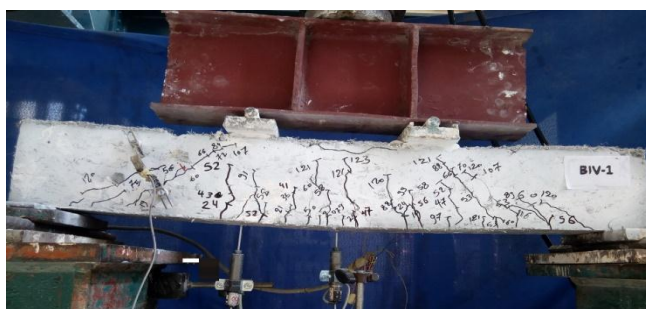
Fig. 10: Final crack pattern of beam BIV-1.
