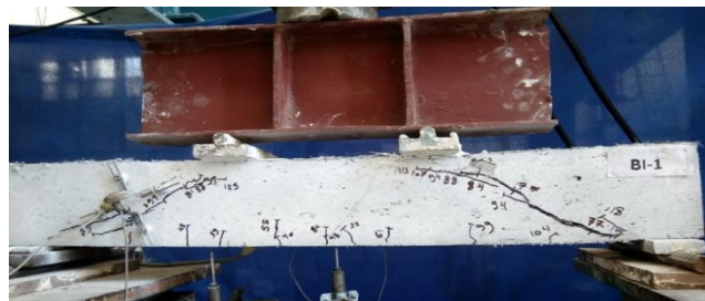
Fig. 7: Final crack pattern of beam BI-1.
