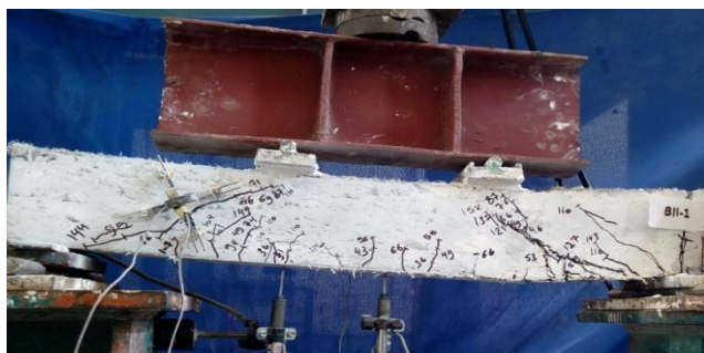
Fig. 8: Final crack pattern of beam BII-1.
