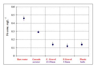
Fig. 7. Changes in Fe concentration after cascade aerator & PBF at different PBF media
