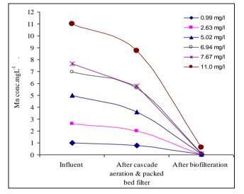
Fig. 10. Mn removal efficiency of the filtration system after each stage.
