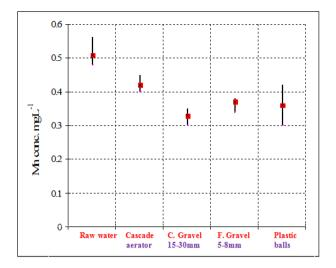
**Fig.** 8. Changes in Mn concentration (mgL<sup>-1</sup>), after cascade aerator & PBF at different PBF media.
