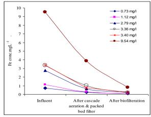
Fig. 9. Fe removal efficiency of the filtration system using after each stage.
