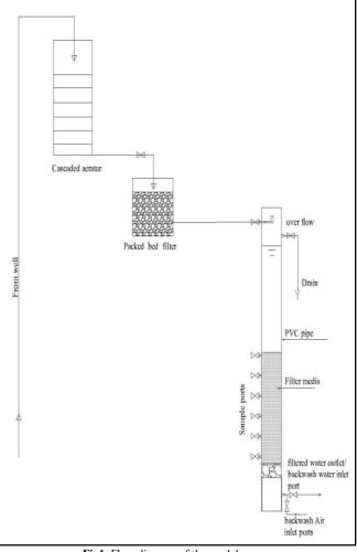
Fig1. Flow diagram of the model.
