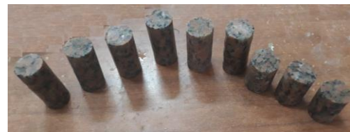
Figure 2. Shape of the Cylindrical Samples of Aswan Granite rocks
