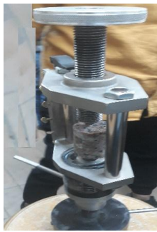
Figure 6. Point Load Test System
