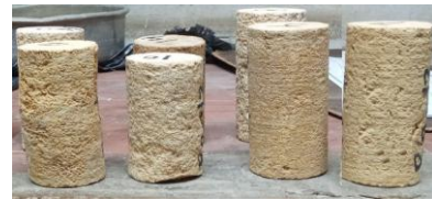
Figure 3. Shape of the Cylindrical Samples of Sandstone rocks
