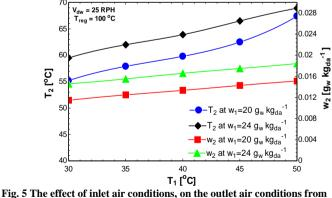
Fig. 5 The effect of inlet air conditions, on the outlet air conditions fro desiccant wheel.
