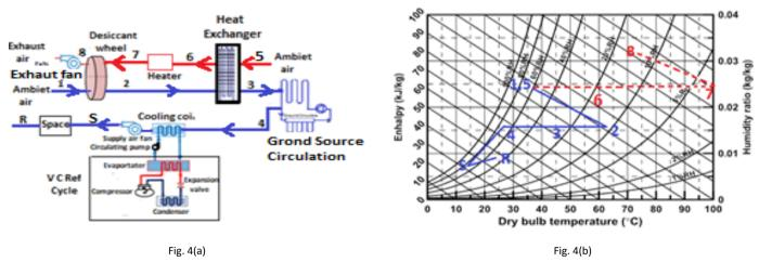
Fig. 4 Central air conditioning system with desiccant wheel / heat exchanger and ground source circulation (system 4). (a) schematic of system, (b) processes of both main air and regeneration air on psychrometric chart.
