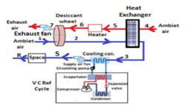
Fig. 2 Schematic of central air conditioning system with desiccant wheel / heat exchanger (system 2).
