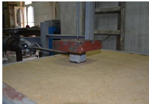
Figure 5. Sample with the Geomembranes.
