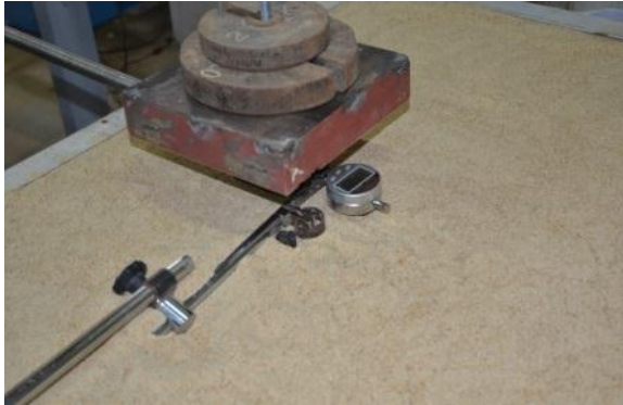
Figure 9. Compacting the Soil.
