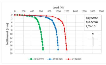
Figure 16. Load-settlement curves for tube piles of 1.5-mm thickness in a dry state.
