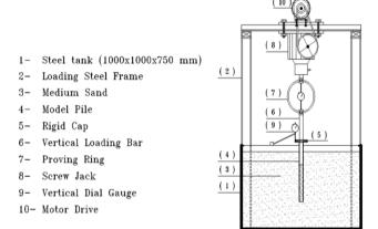
Figure 2. Schematic Diagram for the Model Components.
