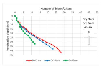
Figure 24. The relation between the number of blows and embedded pile length for different pile diameters at the same pile thickness.
