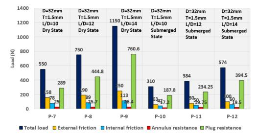
Figure 14. The total pile load with both components is dry and submerged.
