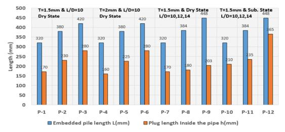
Figure 23. The relation between embedded pile length and plug length inside the pipe
