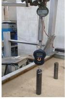
Figure 4. Proving ring with dial gauge 0.002 mm accuracy and a Sensitive balance.
