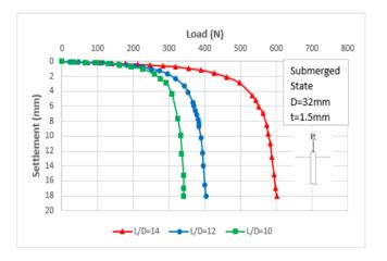
Figure 19. Load-settlement curves for tube piles of different embedded pile lengths, submerged state.
