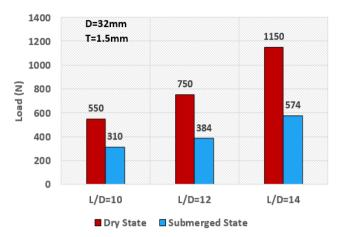
Figure. 20. Effect of Ground Water Table on the Ultimate Pile Capacity for pile diameter 32mm and pile thickness 1.5mm.
