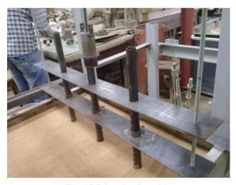
Figure 7. Driven the pile models.
