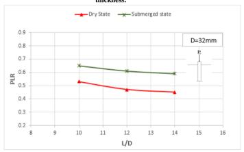
Figure 22. The relation between embedded pile length and plug length ratio (PLR) for dry and submerged states
