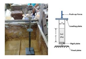
Figure 12. Push-up loading to determine the internal friction for the tube pile.
