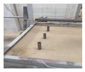
Figure 8. Steel pipe-pile after installation
