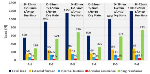
Figure 13. The total pile load with both components is in a dry state.
