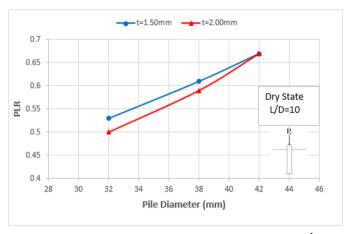
Figure 21. The relation between pile diameter and plug length ratio (PLR) for the dry state, with different pile diameters and different pile thickness.
