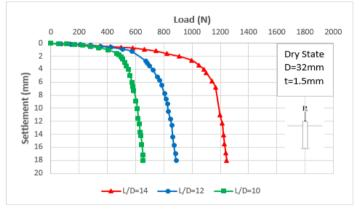
Figure 18. Load-settlement curves for tube piles of different embedded pile lengths, dry state.
