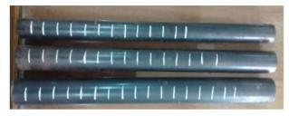
Figure 1. Models of steely tube piles with two different pile thicknesses of (1.5 and 2) mm and pile diameters (32, 38, and 42) mm.
