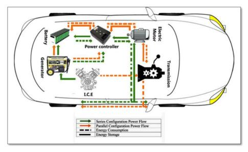
Figure 17. Power flow of a series and parallel hybrid electric vehicle
