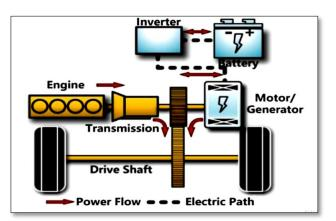
Figure 10. Configuration of parallel HEV [16]
