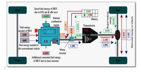
Figure 18. Typical urban cycle energy flows of a conventional powertrain and a hybrid electrified powertrain [19].
