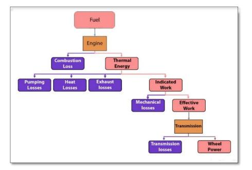
Figure 15. The energy flow distribution and path for conventional vehicles
