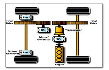
Figure 13. Configurations of subtype P4 in parallel HEVs [16]
