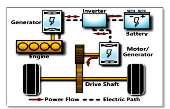
Figure 9. Configuration of series HEV [16].
