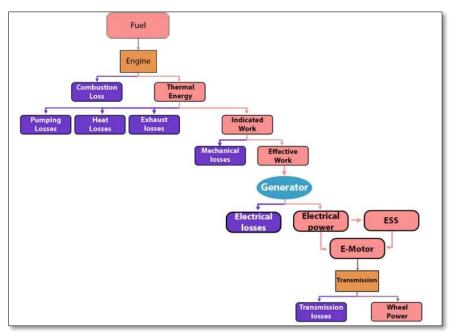
Figure 16. The energy flow distribution and path for PHEV
