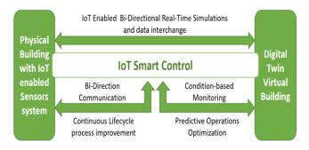
Figure 4. The digital twin concept with the use of IoT to enhance the FM process (by authors)
