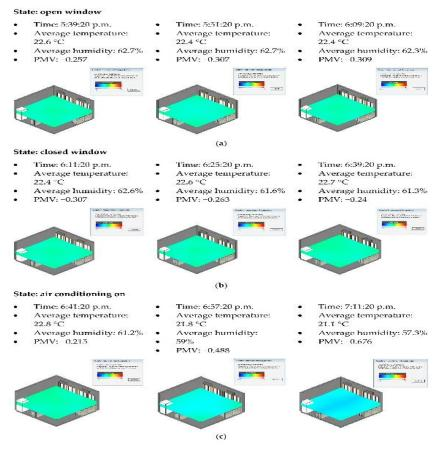
Figure 8. (A) Results of the PMV visualization of the open window condition;
