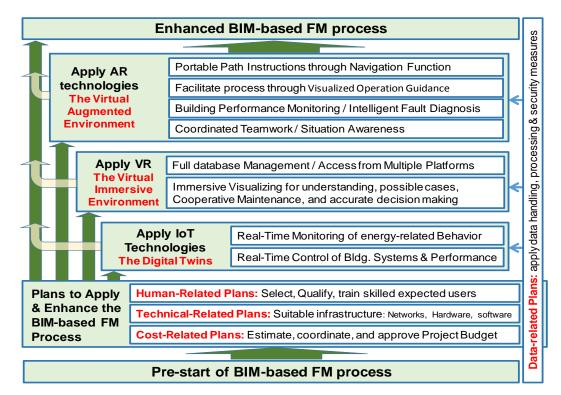
Figure 19. A proposed Framework for integrating IoT, VR & AR with the BIM-Based Facility Management Proces Considering main Benefits and related Challenges (by Authors)
