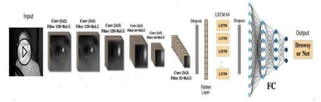
Figure 15. The proposed (CNN-LSTM) model architecture.
