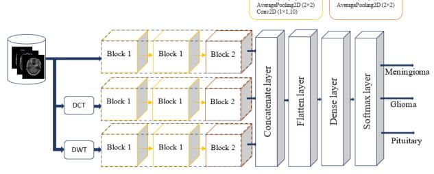
Figure 2. The proposed model for multi-class brain classification.
