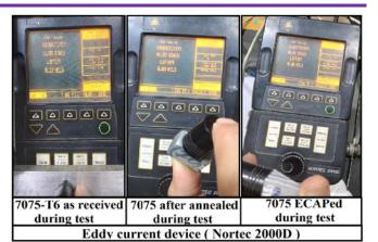
Fig. 9. Nortec 2000 device used to evaluate the electrical conductivity
