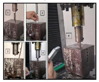
Fig. 4 The billet during ECAP
