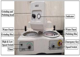
Fig. 7. Spectrum System 1000 (SS-1000) Grinder/Polisher machine
