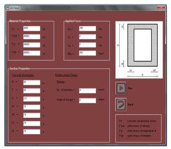
Figure 3. Input data for box section
