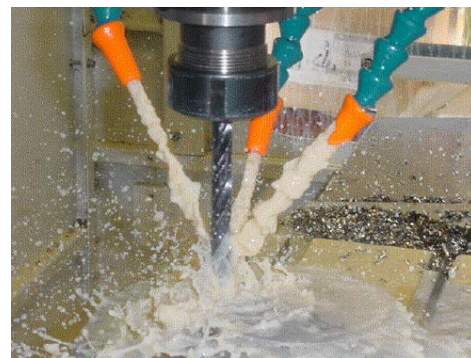
Figure 8. Flood cooling technique [66].
